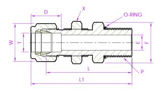
Fractional Tube x SAE/MS Straight (M)
