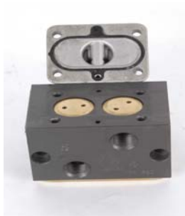
Manual Override Position interchanged for Valve Type 52400 Photo – 8
